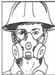
Cartridge respirator (for low to medium dust levels).
