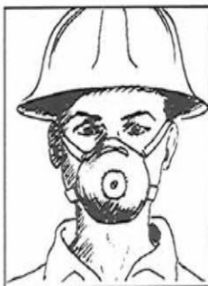
Disposable dust mask (for low to medium dust levels).
