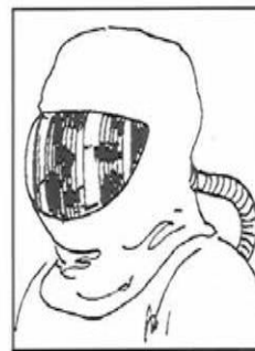
THIS TYPE SUPPLIES CLEAN AIR. Airline hood respirator (for very high dust levels).
