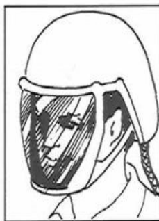
THIS TYPE FILTERS THE AIR. Battery powered respirator (for medium dust levels)
